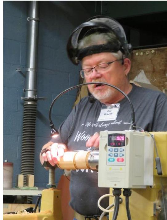
Then part the lid and bottom. Then hollowed the base talking about how to accomplish this without a boring bar. Cut tenon for lid. Then mounted the top, hollowed it and fit mortice to the boom.
