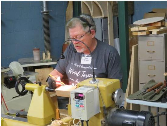
He then turned a small cedar box. Started by rounding a piece of cedar between centers. Showed us his homemade golden ratio caliper. Used it to lay out the box. Turn a tenon on each end to hold in chuck.
