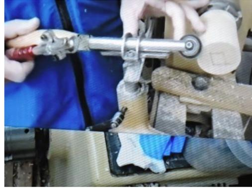
Lathe speed with these tools, however, is more important. For the small toothed tool, he recommends the wood turning at about 450 rpms, and up to 750 rpms with the large toothed tool.
