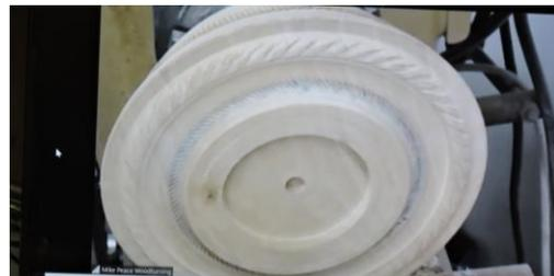
This can also be used to emboss. The burr has to be able to spin against the wood, and this means that it must spin in the tool handle. Mike offers a hand-out to make this tool on his web site, and to make it simpler for you, I have downloaded it and it will also accompany this month's newsletter, also with his permission.
